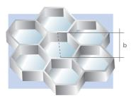
The **honeycomb core** consists of aluminium foils made of the alloy AIMn (EN AW 3003) Cell size b: approx. 6.3 – 12.7 mm. The **cover sheets** of the ALUCORE® panels consist of corrosion-resistant Peraluman alloys (AIMg) and may be used in a decorative or functional manner, depending on the purpose of application.
