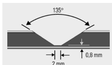
Groove (V-shaped) for edges up to 135°
