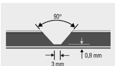
Groove (V-shaped) for edges up to 90°
