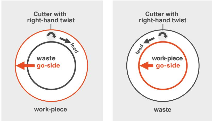
Panel = work-piece, feed in clockwise direction
