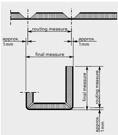
Determination of the routing measure
