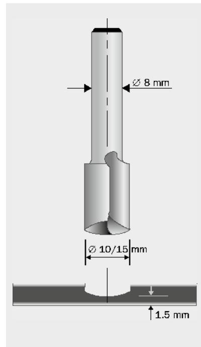
End milling cutter for rectangular grooves
