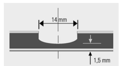
Rectangular groove for edges up to 180° depending on panel thickness
