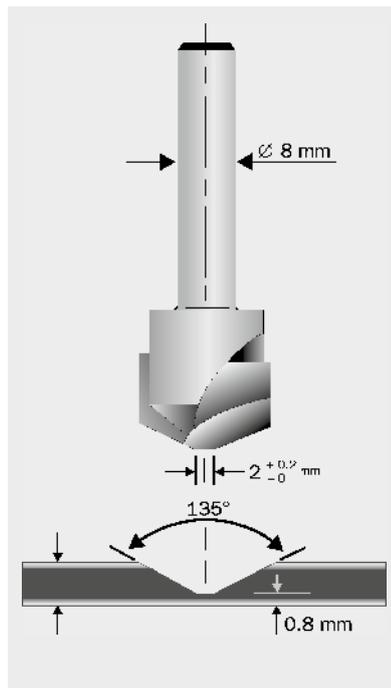
End milling cutter for V-grooves 135°
