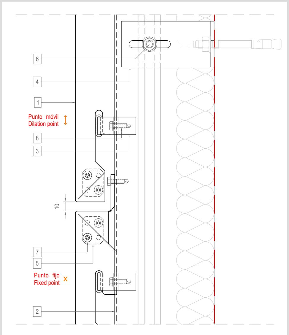
Riveted system - VERTICAL PROFILES
